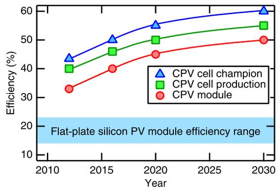
Fig. 1. CPV actual 2012 and targeted 2016, 2020, and 2030 (champion and production) cell and module efficiencies. Flat-plate silicon efficiencies are also indicated.
